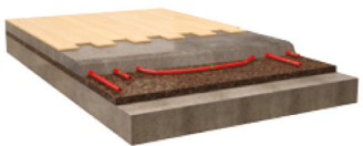
TRADITIONAL UNDERFLOOR HEATING
