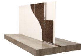
METAL-STUD WALL AND SLAB DISCONTINUITY
