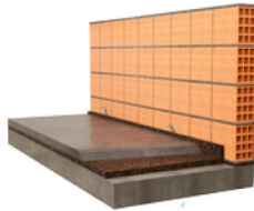
UNLINKING SCREED FILLER TO THE WALL
