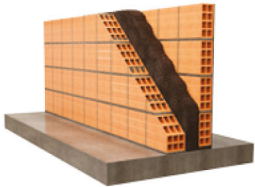
FILLING THE INTERNAL DOUBLE WALLS WITH EXPANDED CORK GRANULES
