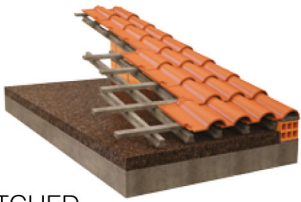
PITCHED ROOF WITH RIGID INSULATION OVER SLAB
