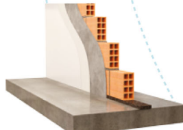
MASONRY WALL AND SLAB DISCONTINUITY
