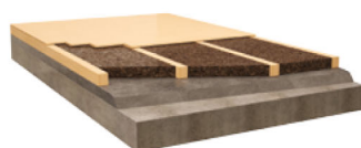
FLOORING JOISTS CAVITY FILLING
